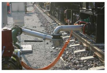
the left shows a loading arm where aviation fuel is being unloaded from railway wagons for transportation by pipeline to Arlanda airport. We manufacture three types of **Loading Arms:**
